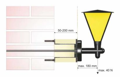
There is necessary to cut the carrier including inserted insulation before installation depending on layer thickness insulation.
